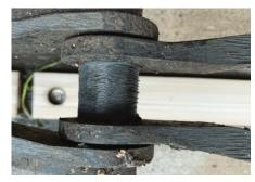
The deep scoring on the barrel of this chain is evidence of grit intrusion. Although still within tolerance, the wear rates will be accelerated and need to be monitored closely.
