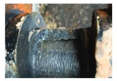
This is a heavily worn chain with the pin almost through the barrel. It will soon fail in the same way that the "beyond failure point" link did with a complete system failure ensuing.
