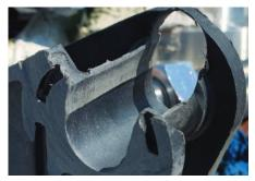
This attachment link has a chain pin which has worn completely through the barrel and consequently cause a complete chain failure.
