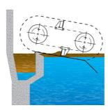
A power skimmer is a 2 or 3-shaft chain and flight system designed to remove grease, scum and other floating materials f om the surface. Similar to 2, 3, and 4-shaft sludge collector systems, the power skimmer is operated by a gear motor, which translates rotation to collector sprockets to drive the chain and flight system. Flights transfer he scum up a beach plate through a scraping action and discharge it into a sloped trough. Power skimmers are standardly equipped with nonmetallic components.
